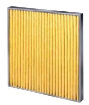
AmAir® HT is designed for applications with continuous operating temperatures up to 500°F (260°C). AmAir HT is rated UL Class 1 with 30-35% average ASHRAE efficiency. The frame is an aluminized steel U-channel, with the media pack bonded to the inside on all four edges. An expanded aluminized steel faceguard is spot welded inside the frame on the air leaving side to retain the media pack at elevated temperatures. AmAir HT is made with microglass media.
