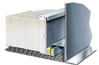
AAF gel sealant in a pocket along the perimeter of the AstroCel® II filter cartridge forms an airtight seal.
